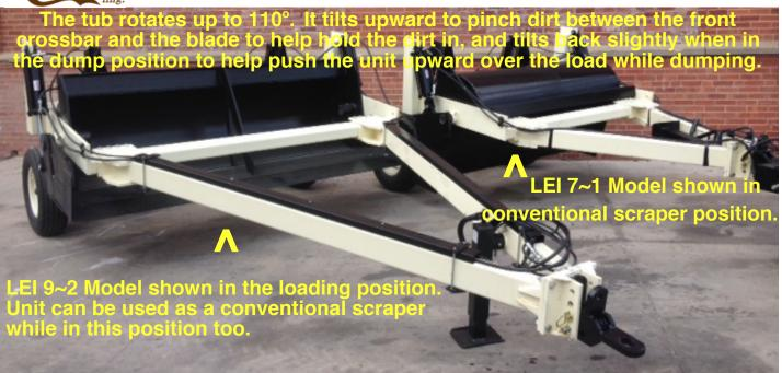
LEI scrapers are available in three different sizes: shown ^ 7~1 which is 7' wide; carries about \*1 yard of dirt. shown ^ 9~2 which is 9' wide; carries about \*2 yard of dirt. 11~3 which is 11' wide; carries about \*3 yard of dirt. 13~4 which is 13' wide; carries about \*4 yard of dirt.
