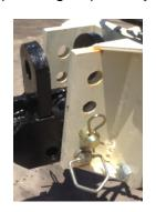
Each unit comes with an adjustable and replaceable front hitch that has many options to choose from.
